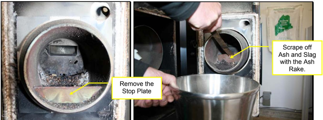
Remove the stop plate from the combustion chamber tube and scrape off ash and slag with the supplied ash rake. Check that the air holes in the combustion chamber tube are free from residuals.
