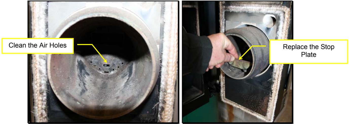
Remount all components in reverse order. Remember to replace the stop plate. Connect the control box cable before connecting the main power supply and auger power cable. Reconnect the pellet feed hose from the pellet feed tube / flame trap pipe.
